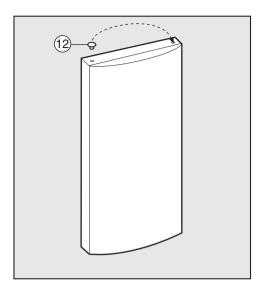
■ Remove cap ② from the bearing bush in the door and refit on the opposite side.
